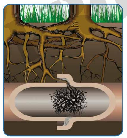
Roots enter through cracks in your underground plumbing lines and cause major clogs.
